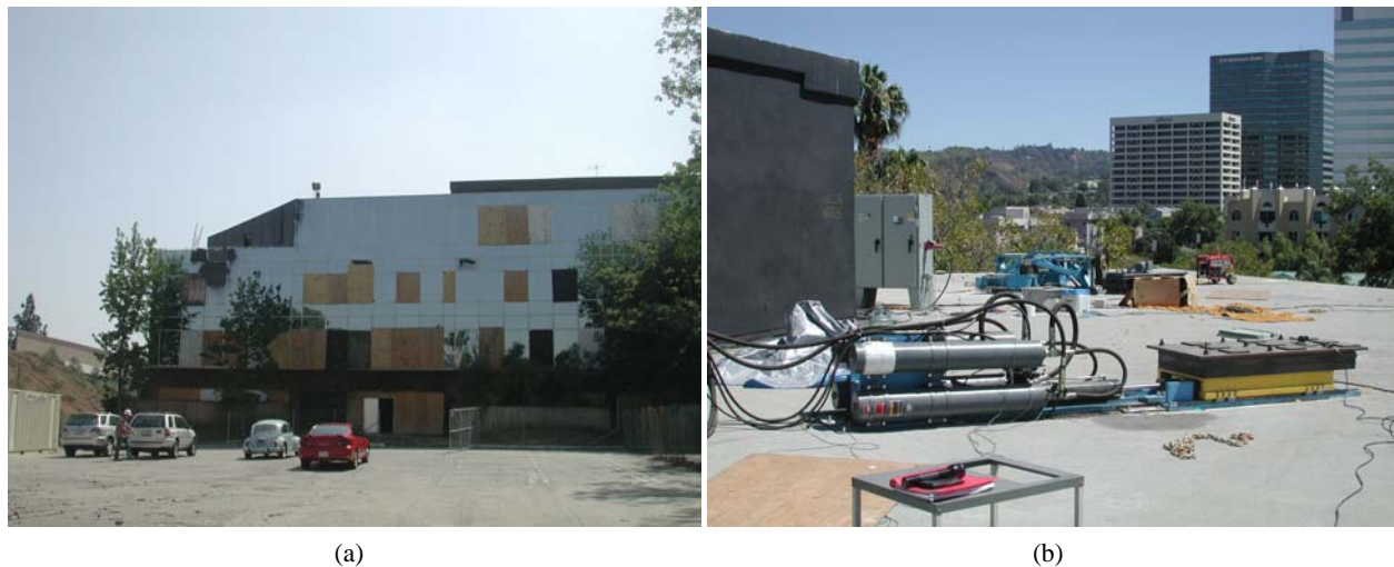
Figure 2. The Four Seasons building: (a) photograph of exterior of building and (b) photograph of two shakers mounted on the roof of the building (linear shaker shown in the foreground, eccentric shaker in the background).
